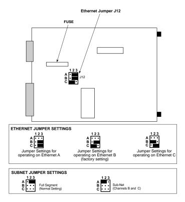
Figure 2-1 CSMIM-T1 Jumper Settings
